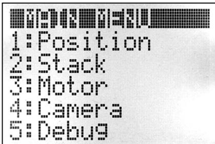
From the main menu, press the digit on the remote which corresponds to the desired task. If you have just assembled the stacking controller or installed updated software, go to the motor configuration ("Motor") and camera configuration ("Camera") menus to set up the controller as desired.
