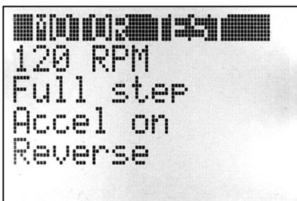
The test motor feature will automatically test your stepper motor using multiple combinations of settings and will measure the actual RPM against several target RPM settings. If you make changes to the code in the stepper motor library, use this feature to test whether the code is functioning correctly.
