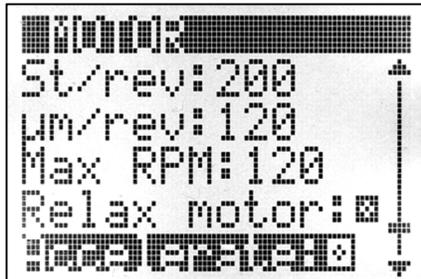
The motor configuration menu allows you to adjust the behavior of the stepper motor and provide the stacking controller with the information necessary to calculate stack depth.
